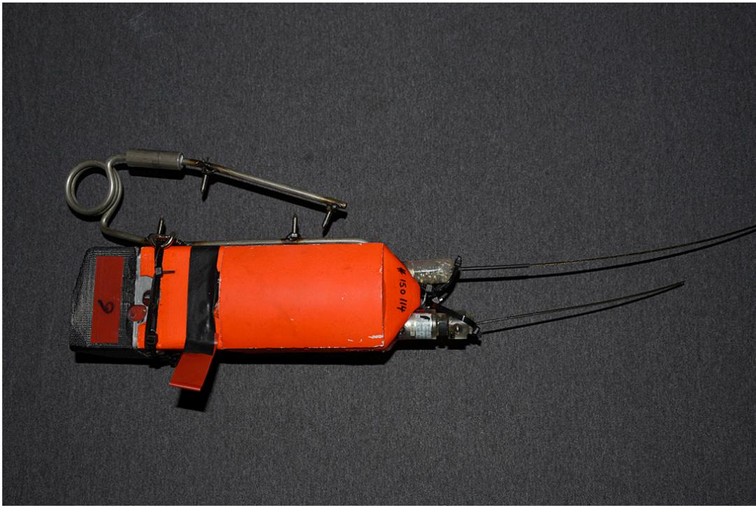
**Figure 6.** CATSCam camera tag with fin bracket, SPOT6 satellite tag and VHF pinger for location and retrieval. (Jonathan R. Green FMME/GWSP/DPNG).
