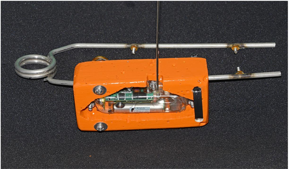
**Figure 6.** Fin mount SPOT6 prototype previously deployed on juveniles. (Photo:©Jonathan R. Green 2017).
