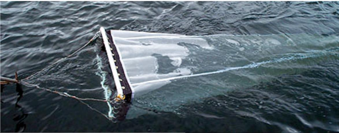
**Figure 11.** Neuston net for plankton and micro plastic tows
